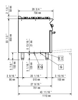
Electrical inlet (power) Gas connection
